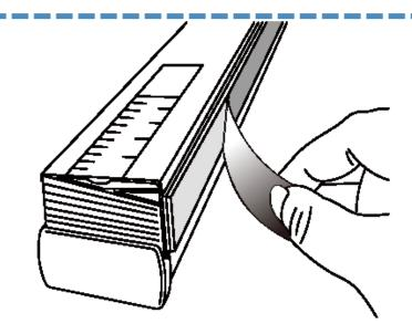
2. Tape the double-sided tape to the top of the headrail.
