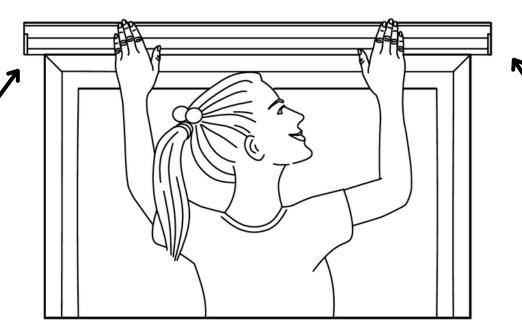
3. Attach the shade to the wall above the window frame.
