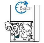
Repeat steps 1-6 for all motors. Once complete Press and hold the Lock button for 6 seconds while looking at the LED, and hold until solid.
