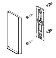
Replace cover by pressing snap latches into place.
