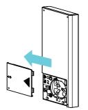
Remove cover from remote; unscrew with screw driver then firmly press down and slide left.
