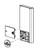
Install battery CR2430 with positive (+) side facing up.
