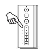
Press any ch to see previously selected channels. The last selected channel will remain in memory. To un-select a channel press the same channel and select any new channels.
