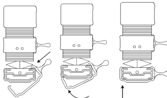
For shades  $W \leq 38''$ , single cordless handles should be operated from the center of midrail and bottomrail.
