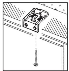
Make sure both brackets are aligned. "L" shape opening should be facing down, with longer side against top of the window opening.
